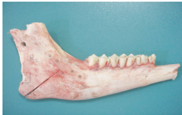
Fig. 2. A single 4-hole absorbable plate (PLLA + PLDLA).
