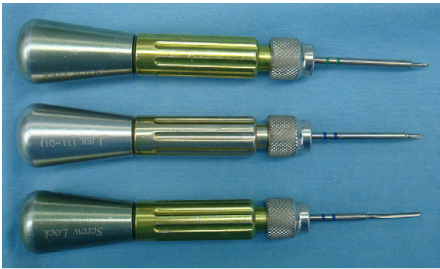
Figure 1 1.5 and 2 mm sized thread-tappers.
